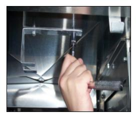
Removing bracket (bottom view)
